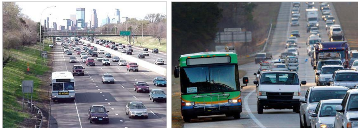
FIGURE 3-25 | MINNEAPOLIS AND RALEIGH, NC BUS-ON-SHOULDER OPERATIONS
