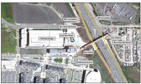
At other locations, the bus stops have been developed along the interchange ramps. At McCaslin, the bus stops have been developed on the southbound off-ramp and the northbound on-ramp. This configuration requires buses to exit the freeway and to travel through the traffic lights at the ends of the freeway ramps. This operation is slower than the exclusive slip ramps in Broomfield, but still fairly direct.
