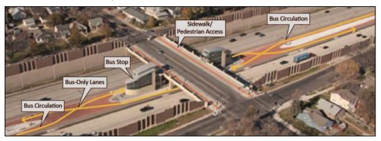
This station was constructed within a narrow median and uses center platforms to reduce the station width. However, most buses only have doors on the right side, which is the wrong side for typical center platform operations. To deal with this issue, once within the bus-only area, buses cross over to the left side so that they can board and alight passengers through their right-side doors.
