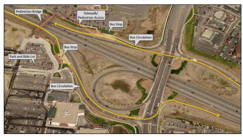
As in Broomfield, this station has a pedestrian bridge that provides access across the freeway and to the park-and-ride lot. Also, RTD is planning to develop bus queue jump lanes along the interchange ramps to reduce intersection delays.
